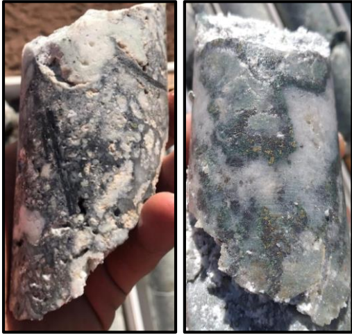
BAN19-209 214.6 to 215.6m at 3,169 gpt AgEq BAN20-243 253.5 to 255.5 m at 13,345 gpt AgEq
