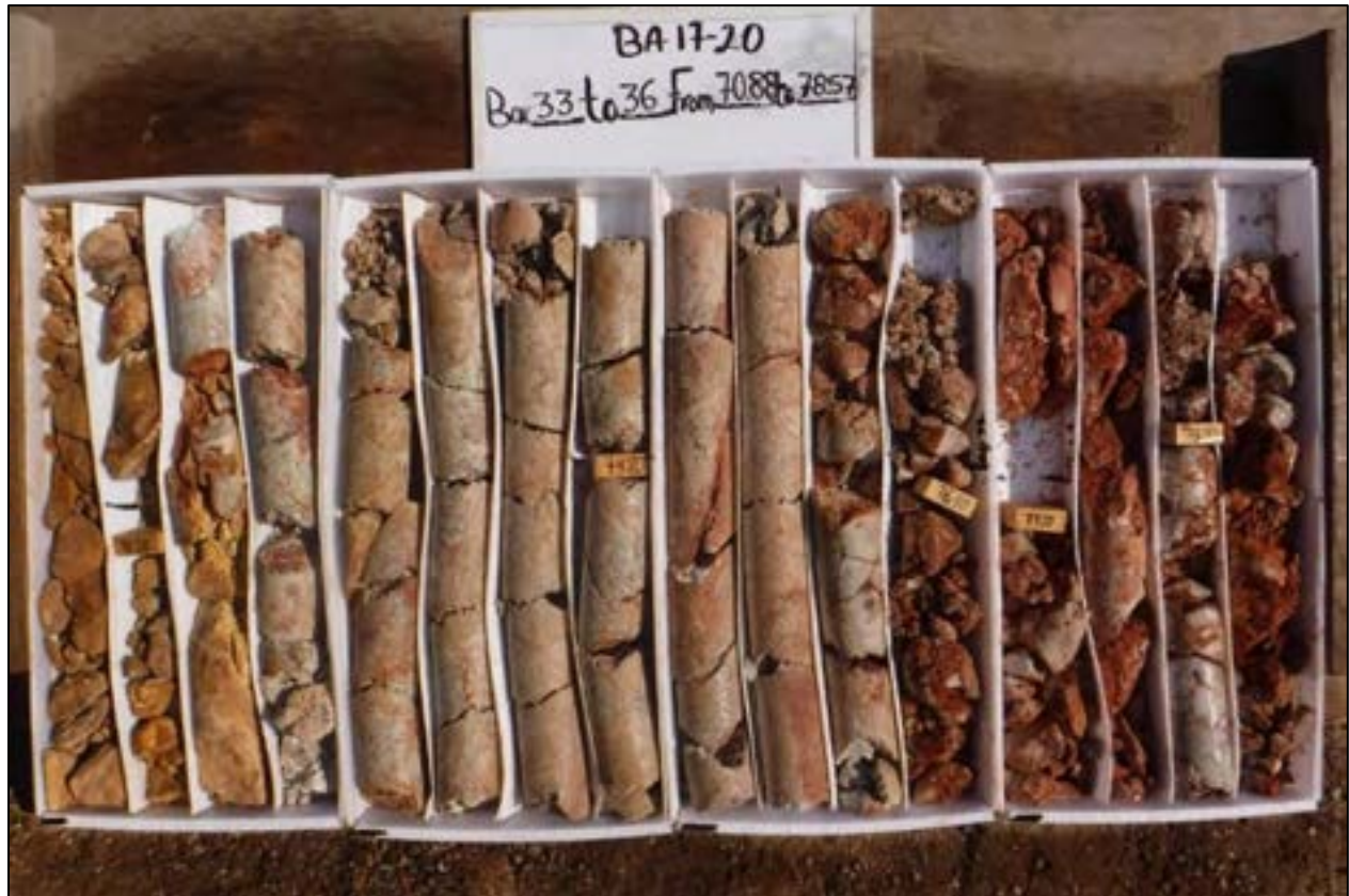
Photo 6-14: DH BA-17-20, from 75.7 m to 78.2 m Grading 3.05 gpt Au and, 77.8 gpt Ag, or 306 gpt AgEq
