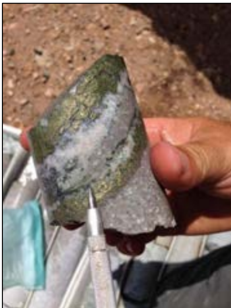
Photo 6-15: Drill Hole GR-17-02; from 139.85 m to 140.55 m, 0.7 m Grading 8.15 gpt Au and 387 gpt Ag, or 998 gpt AgEq, and 1.02% Cu
