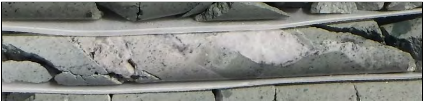
Photo 6-13: Drill Core, LC-17-61 at La Blanquita, 116.0 to 116.55 m, 6.65 gpt Au and 1445 gpt Ag, or 1943 gpt AgEq in a Saccharoidal-Comb Quartz Vein
