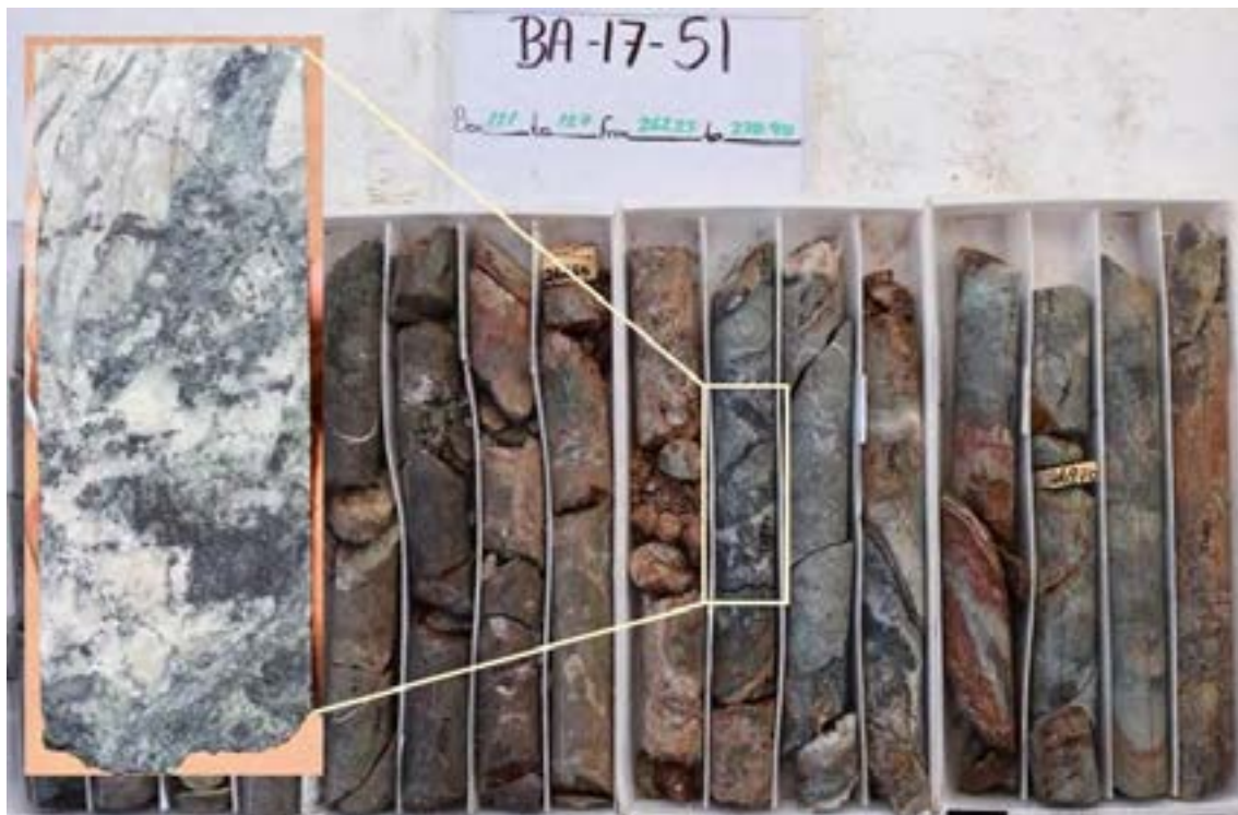
Photo 6-6: Area 51 Mineralization, Babicanora Hole BA17-51 (Discovery Hole); from 265.9 to 269.2m, 3.3 (3.1m true width) metres grading 40.45 gpt Au and 5375.2 gpt Ag, or 8409 gpt AgEq, with hematite breccias, coarse banded argentite, native silver, electrum and native gold.
