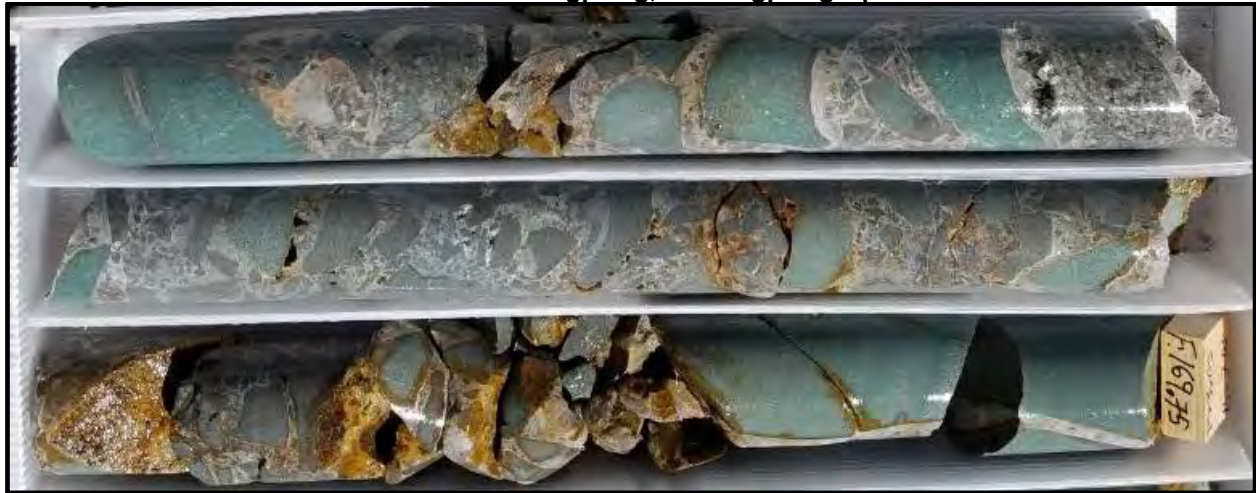
Photo 6-11: Drill Hole LC-17-69; from 168.2 to 169.75 m, includes 1.6 m True Width, Grading 1.95 gpt Au and 252.0 gpt Ag, or 398 gpt AgEq
