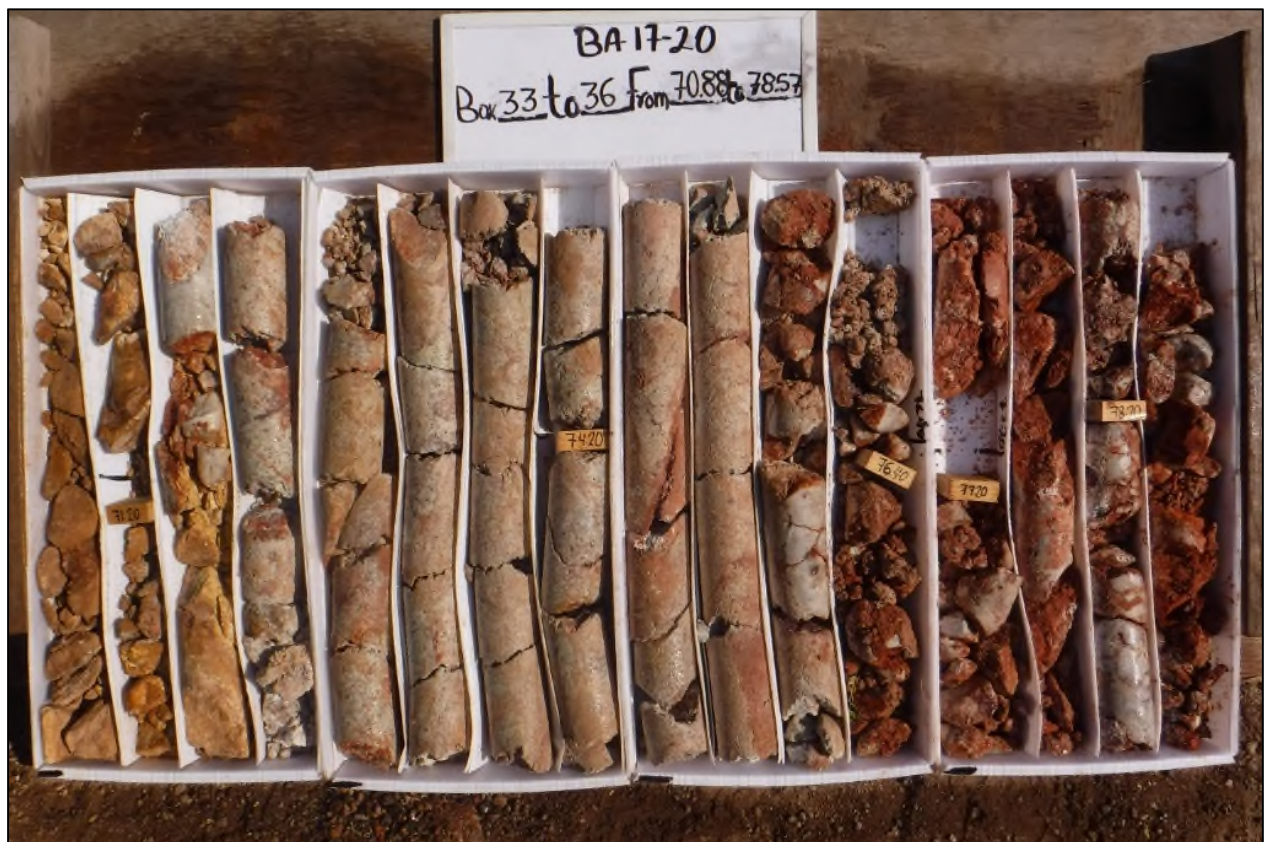
Photo 6-13: Drillhole BA-17-20, from 75.7 m to 78.2 m Grading 3.05 gpt Au and, 77.8 gpt Ag, or 306.55 gpt AgEq
