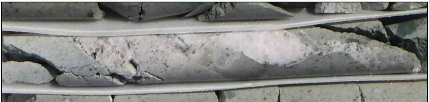
Photo 6-12: Drill Core, LC-17-61 at La Blanquita, 116.0-116.55 m, 6.65 gpt Au and 1,445 gpt Ag, or 1,943.8 gpt AgEq in a Saccharoidal-Comb Quartz Vein
