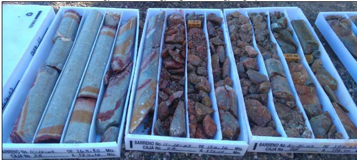
Photo 6-9: William Tell Vein, drillhole LC16-03; from 172m to 176m, 4m (1.5m true width) grading 2.03 gpt Au and 683 gpt Ag, or 835.25 gpt AgEq
