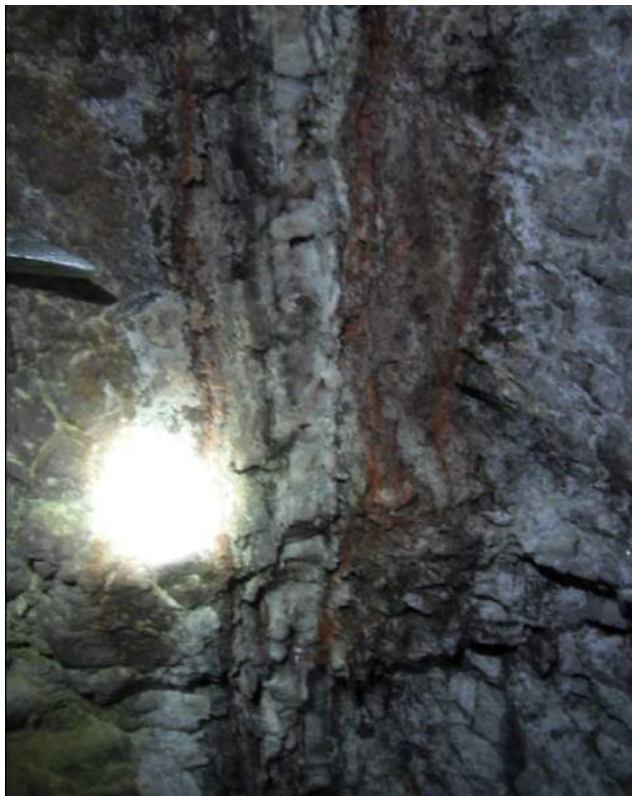
Photo 6-2: Laminated (banded) Vein Style Mineralization along Las Chispas Vein, tip of Rock Hammer shown on Upper Left (near SilverCrest sample 227908, 1.04 gpt Au and 197 gpt Ag over 1.33 m)
