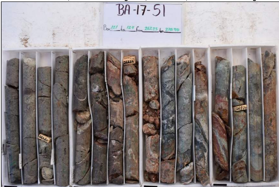
Photo 6-6: Area 51 Mineralization, Babicanora Hole BA17-51 (Discovery Hole); from 265.9 to 269.2m, 3.3 (3.1m true width) metres grading 40.45 gpt Au and 5375.2 gpt Ag, or 8,408.95 gpt AgEq, with hematite breccias, coarse banded argentite, native silver, electrum and visible gold.
