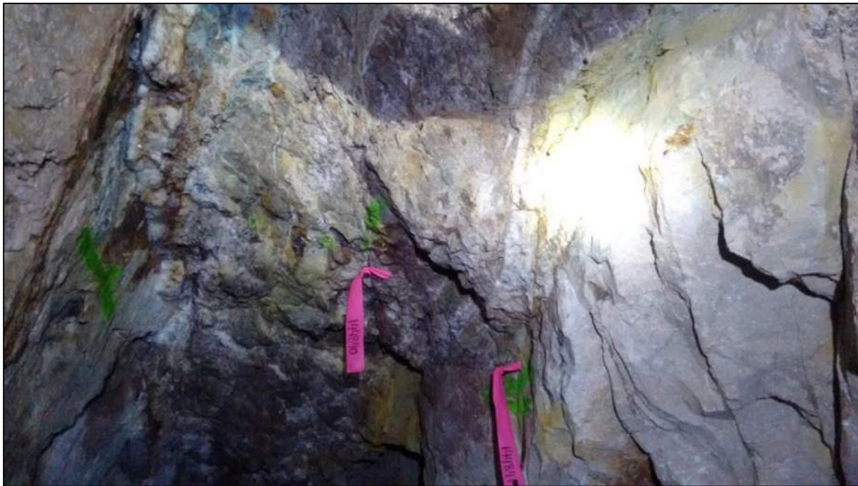
Photo 6-8: William Tell Underground Channel Sample No. 144840 grading 13.4 gpt Au and 1,560 gpt Ag, or 2,565 gpt AgEq
