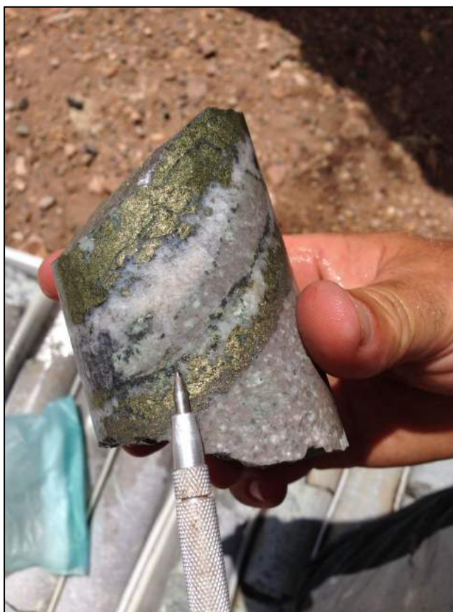
Photo 6-14: Drillhole GR-17-02; from 139.85 m to 140.55 m, 0.7 m Grading 8.15 gpt Au, 387 gpt Ag (998.3 gpt AgEq) and 1.02% Cu
