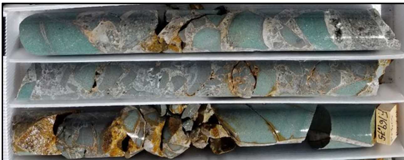
Photo 6-10: Drillhole LC-17-69; from 168.2 to 169.75 m, includes 1.6 m True Width, Grading 1.95 gpt Au and 252.0 gpt Ag, or 398.25 gpt AgEq
