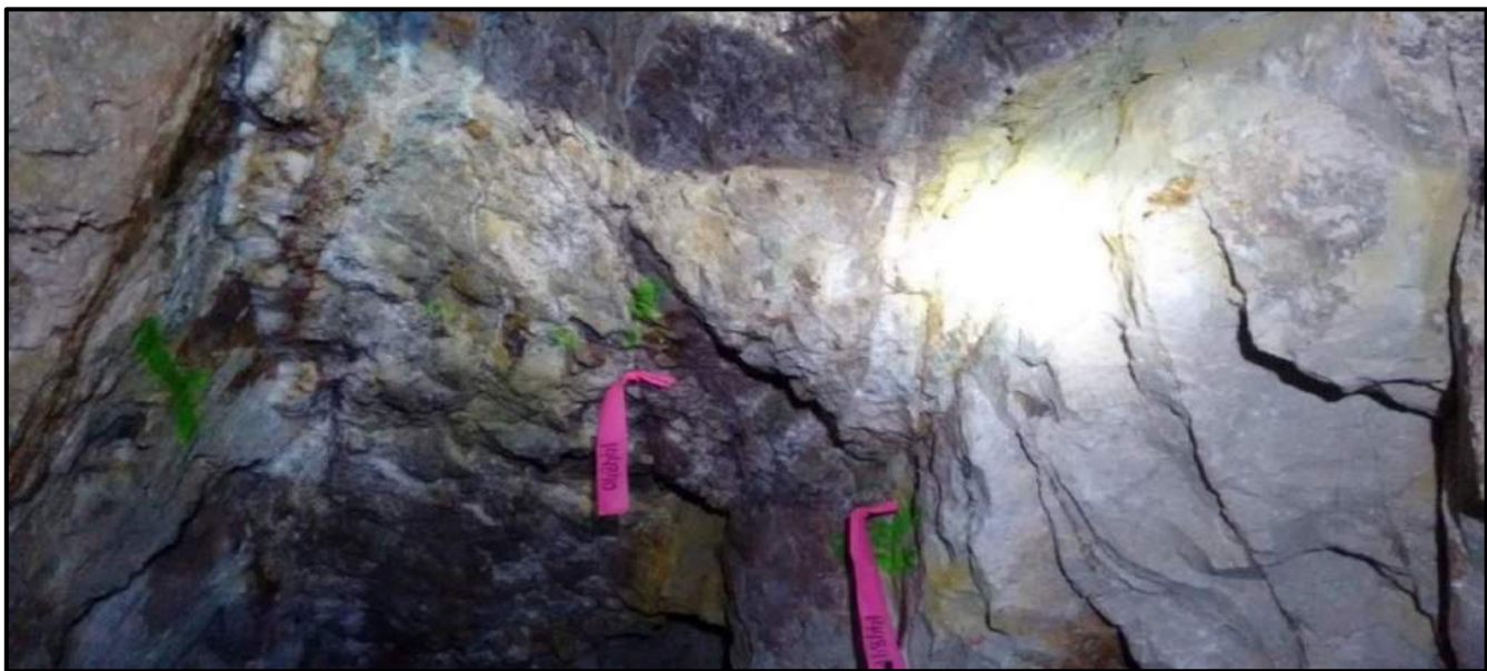
Figure 7-33: William Tell Underground Channel Sample No. 144840 Grading 13.4 gpt Au and 1,560 gpt Ag
