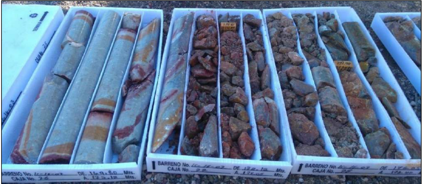
Figure 7-34: William Tell Vein, Drill Hole LC16-03, from 172 to 176 m, 4 m (1.5 m True Thickness) Grading 2.03 gpt Au and 683 gpt Ag
