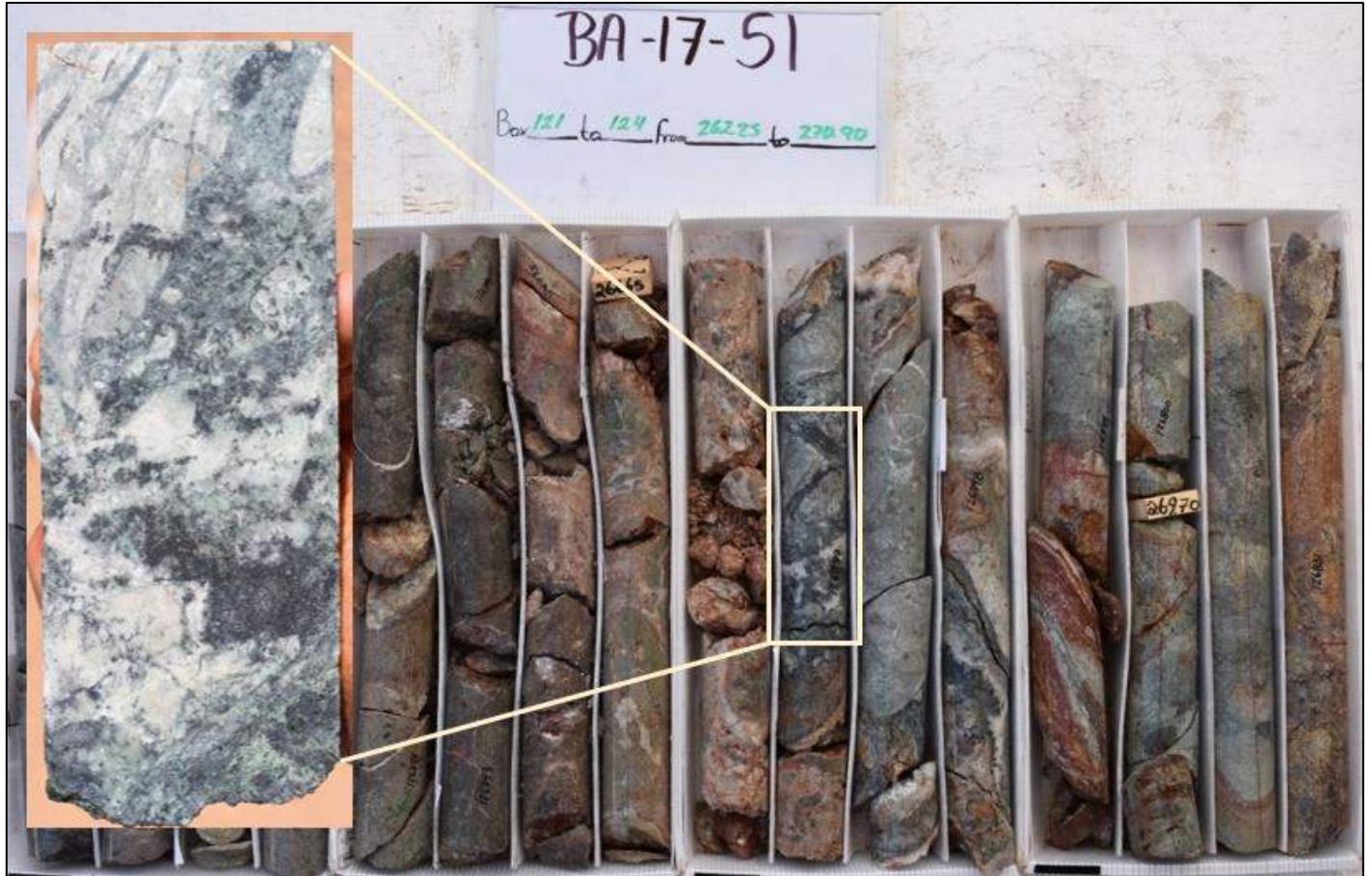
Figure 7-18: Drill Hole BA17-51 (Discovery Hole for Area 51 Zone); from 265.9 to 269.2 m, 3.3 m (3.1 m True Thickness) Grading 40.45 gpt Au and 5,375 gpt Ag, with Hematite Breccias, Coarse Banded Argentite, Native Silver, Electrum, and Native Gold.
