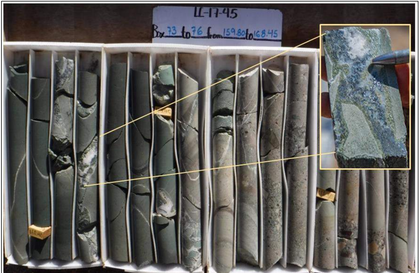
Figure 7-29: Drill Hole LC17-45; from 159.6 to 161.9 m at 2.3 m (1.9 m True Thickness) Grading 50.56 gpt Au and 5,019 gpt Ag with Coarse Argentite and Electrum
