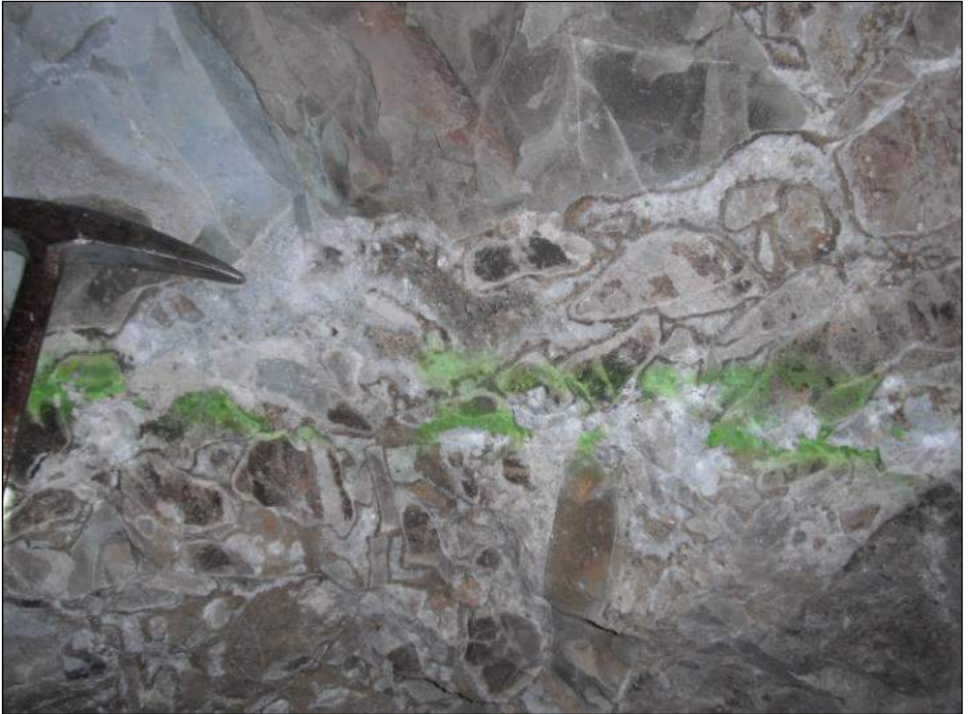
Figure 7-8: Breccia Style Mineralization Along Las Chispas Vein (Base of Las Chispas Gallery near SilverCrest Sample 617179 2.34 gpt Au and 344 gpt Ag)
