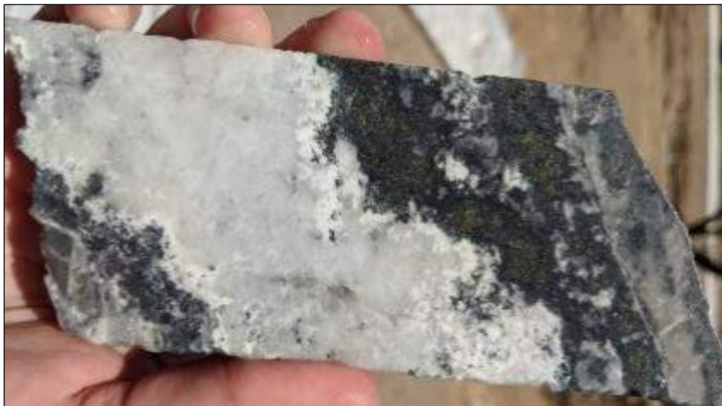
Figure 7-22: Drill Hole BAN18-10, From 93.0 to 95.5 m Grading 61.36 gpt Au and 2,834 gpt Ag with Visible Argentite, Pyrrargyrite, Electrum, Native Silver, and Native Gold
