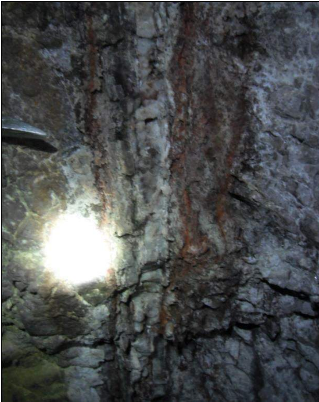
Figure 7-7: Laminated (Banded) Vein Style Mineralization Along Las Chispas Vein, Tip of Rock Hammer Shown on Upper Left (Near SilverCrest Sample 2277908, 1.04 gpt Au and 197 gpt Ag over 1.33 m)
