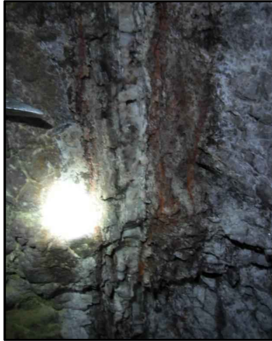
Photo 7-4: Laminated (Banded) Vein Style Mineralization Along Las Chispas Vein, Tip of Rock Hammer Shown on Upper Left (Near SilverCrest Sample 227908, 1.04 gpt Au and 197 gpt Ag over 1.33 m)
