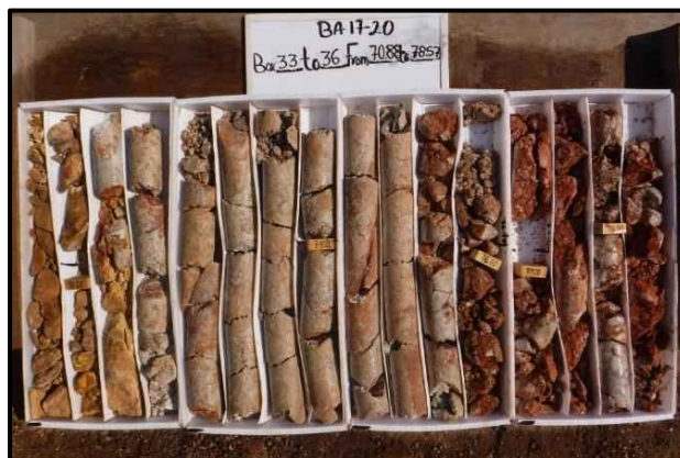
Photo 7-22: Drill Hole BA17-20, from 75.7 to 78.2 m Grading 3.05 gpt Au and, 77.8 gpt Ag, or 306 gpt AgEq
