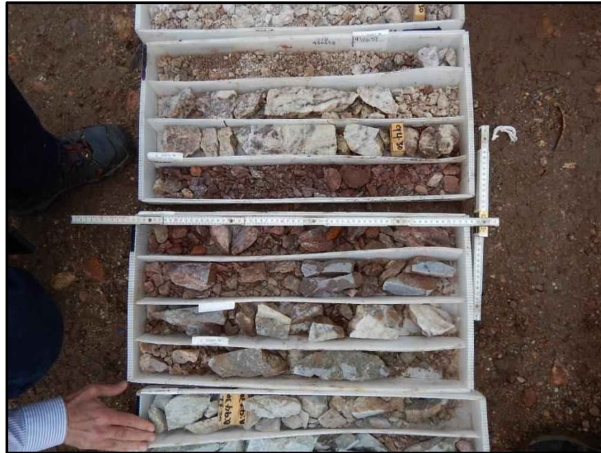
Photo 16-2: Core Box Showing Good Host Rock with Less Competent Rock Within the Mineralized Zone
