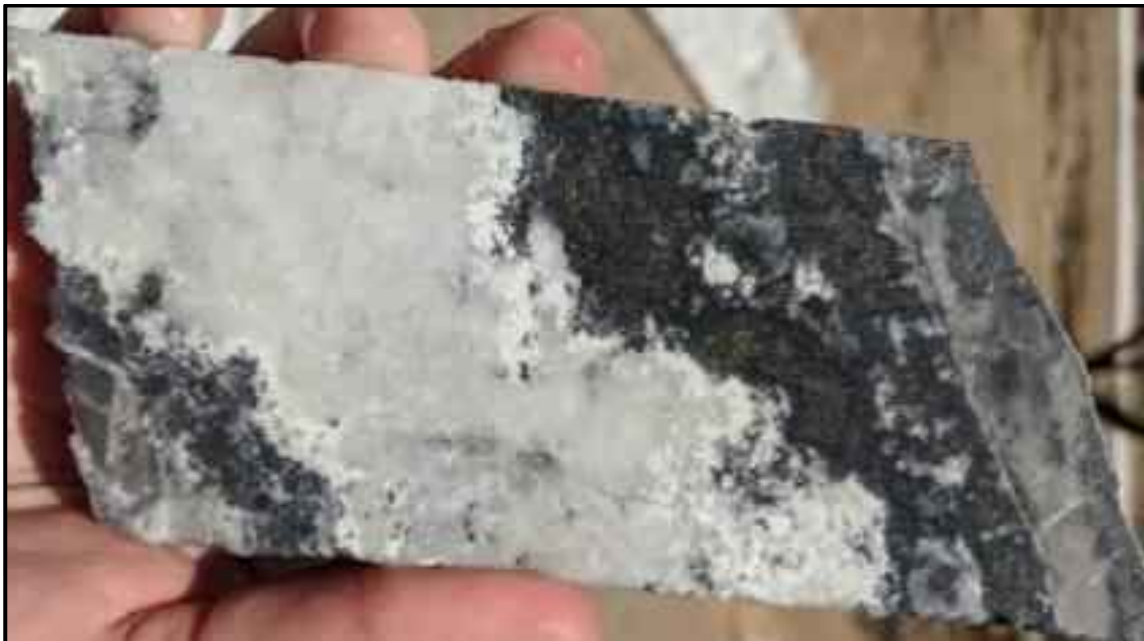
Photo 7-12: BAN18-10, From 93.0 to 95.5 m Grading 61.36 gpt Au, 2,833.5 gpt Ag or 7,436 gpt AgEq with Visible Argentite, Pyrrargyrite, Electrum, Native Silver, and Native Gold
