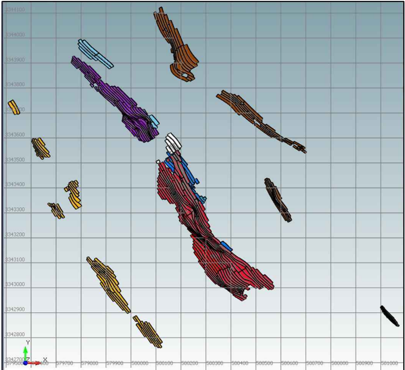
Figure 16-7: Babicanora Final Stopes (Plan View)
