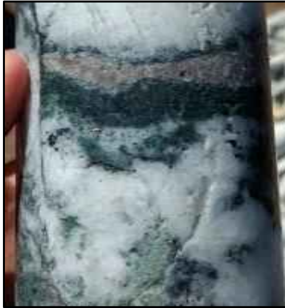
Photo 7-21: Drill Hole GR17-04; from 133.8 to 134.3 m, 0.5 m Grading 47.5 gpt Au and 5,620 gpt Ag, or 9,182 gpt AgEq
