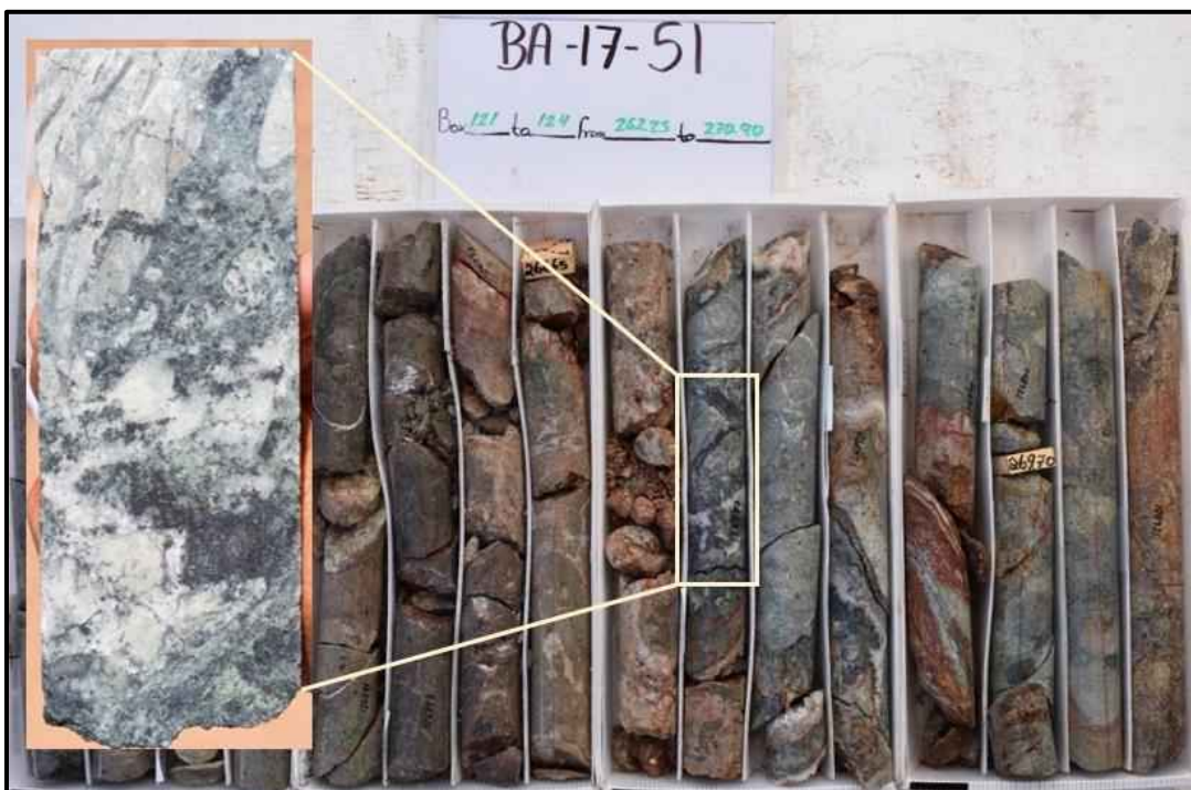
Photo 7-11: Area 51 Mineralization, Babicanora Hole BA17-51 (Discovery Hole); from 265.9 to 269.2 m, 3.3 m (3.1 m True Width) Grading 40.45 gpt Au and 5,375.2 gpt Ag, or 8,409 gpt AgEq, with Hematite Breccias, Coarse Banded Argentite, Native Silver, Electrum, and Native Gold
