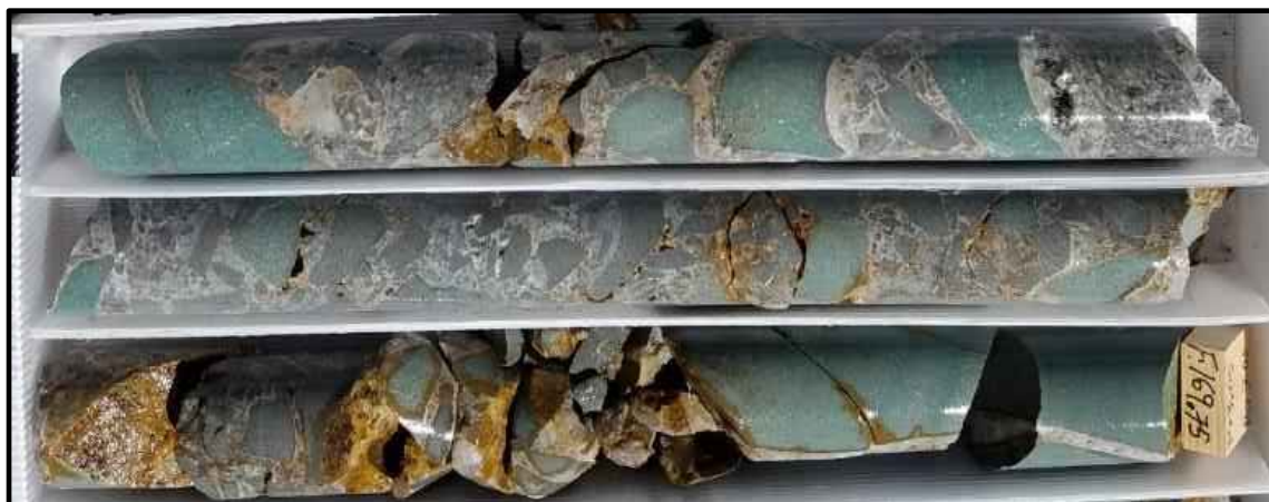
Photo 7-17: Drill Hole LC17-69; from 168.2 to 169.75 m, includes 1.6 m True Width, Grading 1.95 gpt Au and 252.0 gpt Ag, or 398 gpt AgEq
